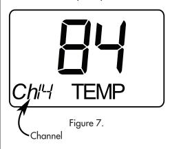
4. The Remote Sensor Screen will display the ambient temperature and, in the bottom-left corner, a channel number between 0 and 15. See Figure 7. This will be the channel to which you will set the thermostat to read the Remote Sensor. See the Thermostat Instruction Manual, page 14, Option 8.
